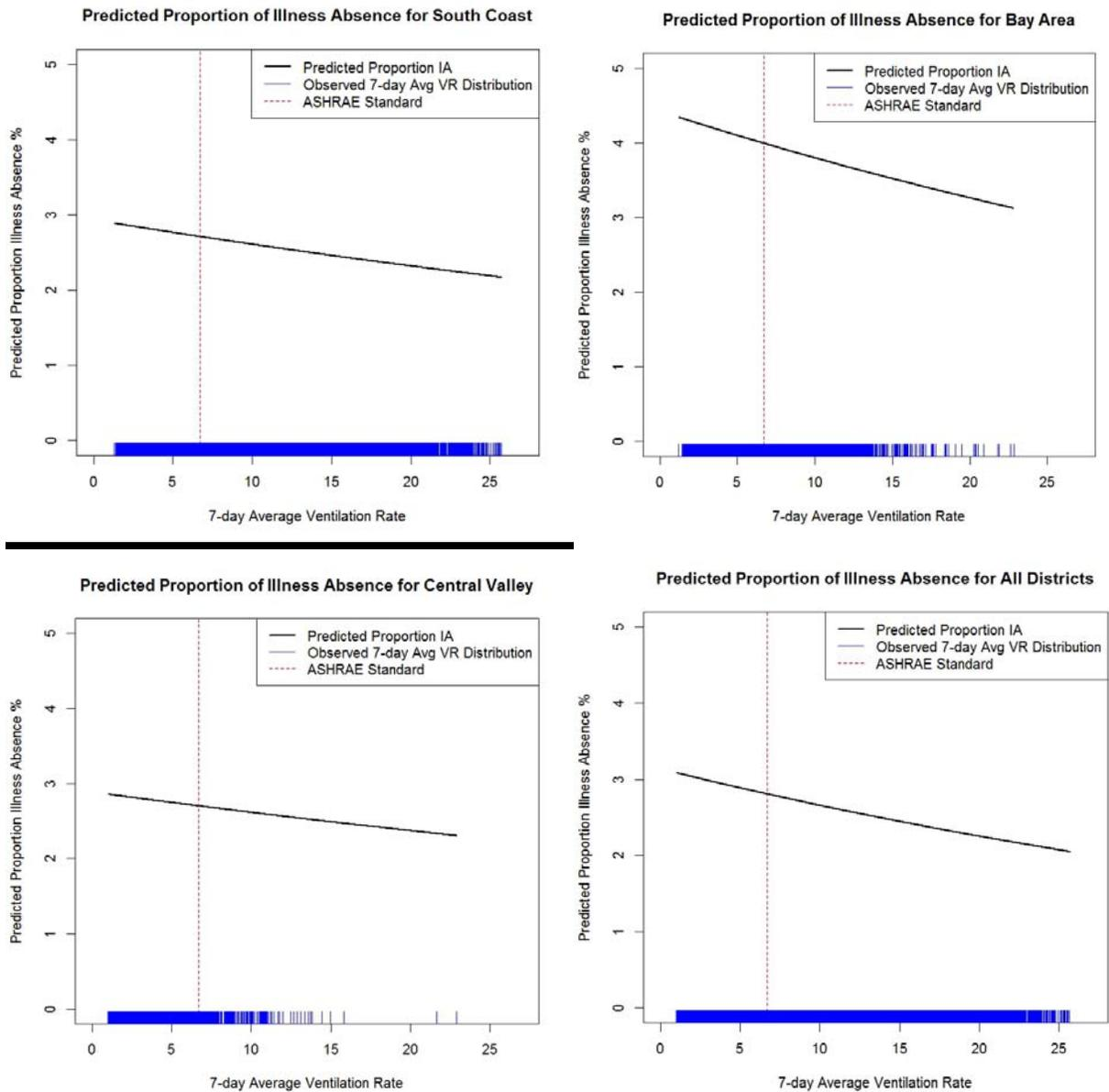
**Figure 3. Predicted relationship between ventilation rate and proportion illness absence in three California school districts** (Vertical bars at the base of each plot shows the VR values of data points on which that the plot was based. Predicted values are for a standard classroom: 5th grade, with 26 children enrolled, 52% male, 63% participating in the free or reduced price meals program, on a Monday in the non-winter season.)
